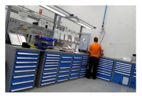
Self-contained tooling hubs serve groups of up to ten machine tools with setting tools, cutting tools and inspection equipment.
