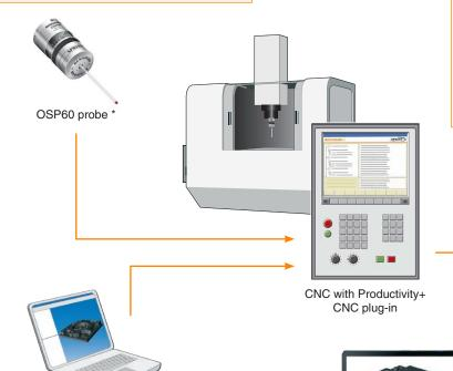
the CNC plug-in resides and operates silently in the background. The operator simply selects the CNC program as usual and the software automatically identifies that CNC plug-in processing is needed. The program then runs with no requirement for operator intervention.
