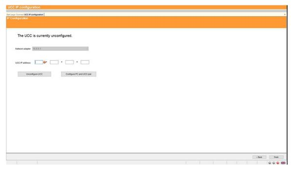
e) Fill in the desired IP address. The IP configuration software has given you a head start by filling in the network part of the address appropriate for the network adapter selected (see section 'IP addressing' for a discussion of the choice and of IP addresses in general).
