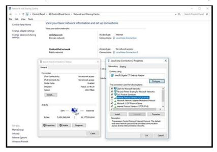
d) Select 'Use the following IP address' and type in the IP address to use for the PC end of the comms link. Click in the Subnet mask field. On Windows10 the Subnet mask will already be filled in. If you have to fill it in for yourself, here are the values:
