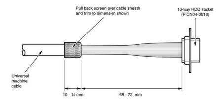
Preparation of Renishaw universal machine cable for shank mounted systems
