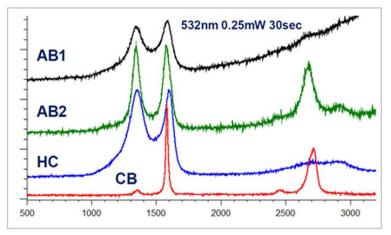
Raman spectra for four different carbon samples, two acetylene blacks (AB), hard carbon (HC), and carbon black (CB). The D-band is at ~ 1350 cm<sup>-1</sup>, the G-band at ~ 1600 cm<sup>-1</sup>
