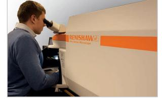
The Renishaw inVia confocal Raman microscope
