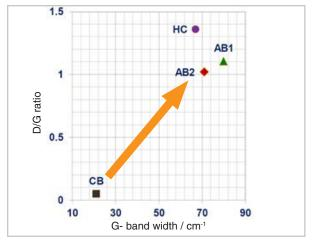
Intensity ratio of the D-band and G-band plotted against width of the G-band. The orange arrow indicates the progression from order to disorder.
