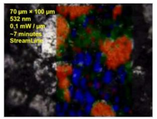
StreamLine Raman image revealing: graphite (red); acetylene black (blue); and hard carbon (green). The relative ratios are: graphite (13%); acetylene black(19%); hard carbon (77%).
