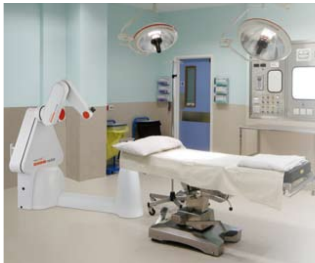
Image guided robotic neurosurgery. The neuro I mate® stereotactic robot is intended to be used in an operating suite for the spatial positioning and orientation of a tool holder or a tool guide in order to guide standard surgical instruments.
