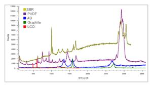
Detecting and identifying all the materials present, even at low concentration. Spectra taken in situ from: SBR (styrene-butadiene rubber, binder); PVDF (polyvinylidene fluoride, binder); AB (acetyl black, anode); graphite (anode); LCO (lithium cobalt oxide, cathode).
