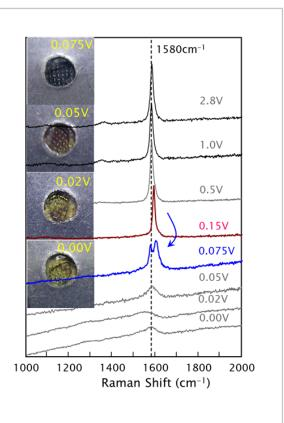
Operando studies of an anode. As the potential is changed, the anode's appearance changes. The graphite G-band Raman peak also changes, indicating intercalation of lithium (shifting the peak to higher wavenumbers) and then a peak-splitting reflecting the intercalation penetrating to interior layers, rather than just the boundary layers. Data courtesy of Prof. Y. A. Kim, Shinshu University, Japan.
