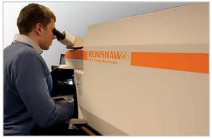
The Renishaw inVia confocal Raman microscope.
