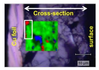
Detecting low concentrations of binder. Raman map of an anode (superimposed on an optical microscope image). The colours represent: SBR styrene-butadiene rubber binder (red); graphite (green); acetyl black (blue). The relative concentrations, as determined by the map, are, respectively: 1%, 97%, and 2%.
