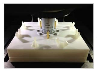
Using an electrochemical cell to perform operando measurements on a lithium-ion battery. Image courtesy of Mr. Hamura, Shimadzu Technoresearch, Japan.
