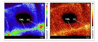
Figure 2. Raman images of cross section of decayed Scots pine wood showing A - lignin concentration changes (intensity changes of Raman band at 1595 cm<sup>-1</sup>), and B - the increased concentration of pinosylvins (Raman band at 1634 cm<sup>-1</sup>).
