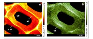
Figure 1. Raman images of cross section of Scots pine wood showing intensity changes of Raman band at 1595 cm<sup>-1</sup> (A, Lignin) and the orientation sensitive cellulose band at 1095 cm<sup>-1</sup> (B, Cellulose).
