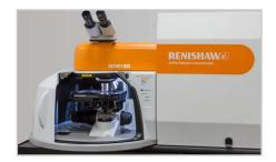
inVia Qontor confocal Raman microscope
