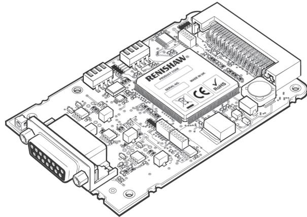
In the VME configuration, no connection is required to the P1 (VME interface) connector; all functions are accessed through the P2 connector.
