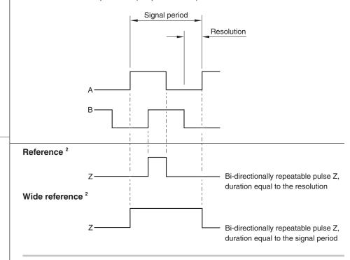
**NOTE:** Select 'standard' or 'wide' reference at time of ordering, to match the requirements of the controller being used.
