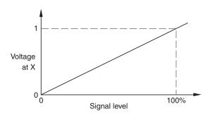
The set-up signal voltage is proportional to the incremental signal amplitude.
