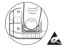
5. Refit the cover plate ensuring the cable ferrule is located in the recess on the inside and no wires are trapped under the cover plate.
