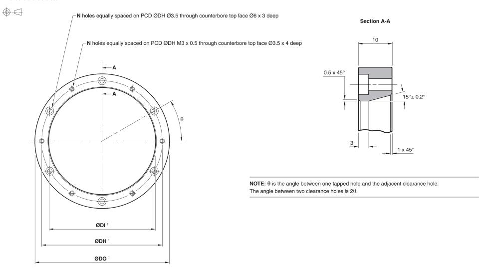
The dimensions DO, DI and DH for the RESM20 'A' section rings are listed on the following page.
