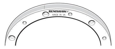
The *IN-TRAC*™ reference mark is integrated in the scale, radially aligned with the centre of the mounting hole to the left of the 'Renishaw' logo within ±0.5 mm. No external actuators or physical adjustment are required.
