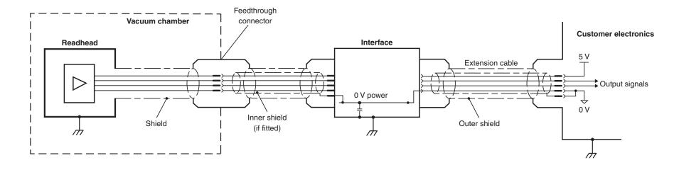
**IMPORTANT:** The outer shield should be connected to the machine earth (Field Ground). The inner shield should be connected to 0 V at receiving electronics only. Care should be taken to ensure that the inner and outer shields are insulated from each other. If the inner and outer shields are connected together, this will cause a short between 0 V and earth, which could cause electrical noise issues.
