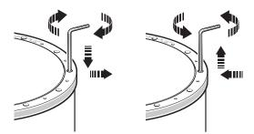
**NOTE:** At this stage, the screws should only be lightly tightened (less than 0.5 Nm) to allow further final adjustment.
